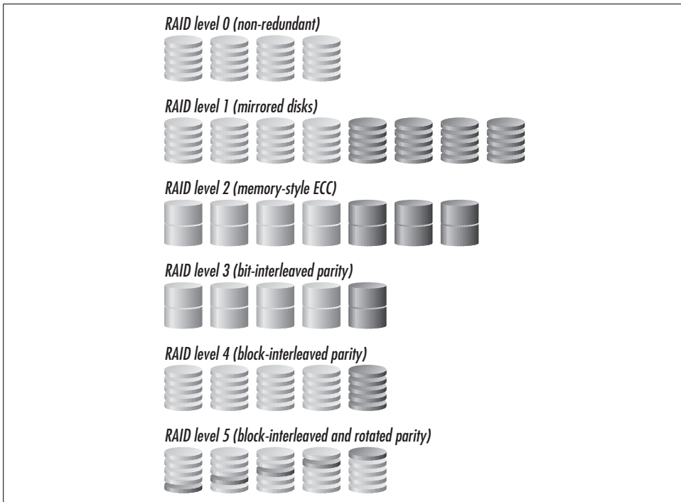
Figure 10-12. Data storage required in the different RAID organizations
